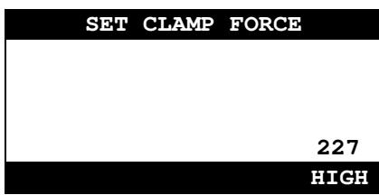
The clamping pressures can be set in the SET CLAMP FORCE menu.
