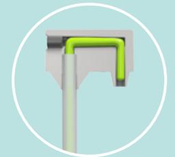
To further reduce adhesions to the drainage rod, the system performs a sniff at the end of every recirculation cycle to eliminate drop formation at the recirculation nozzle.
