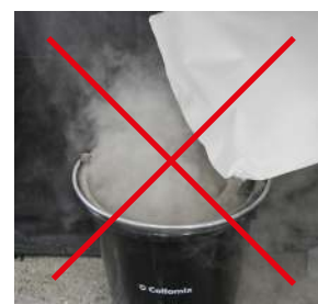
While filling the bucket, a large amount of dust is produced.
